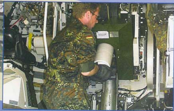
Placement of charge in breech
