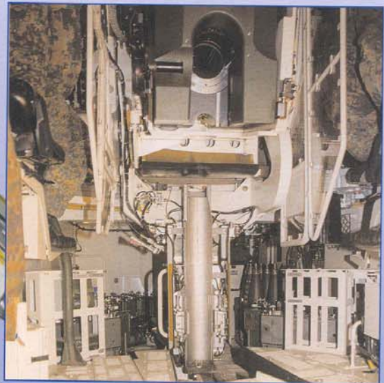
Shell transfer arm with flick rammer
