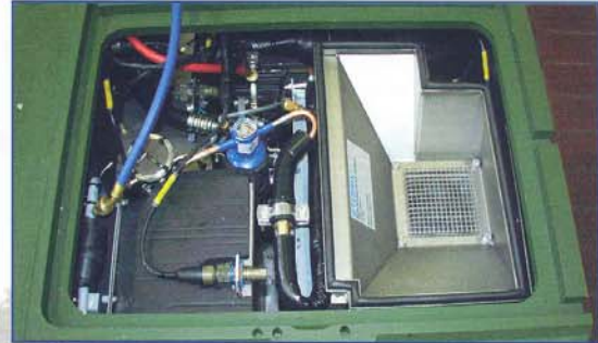
Charge cooling system in turret bustle
