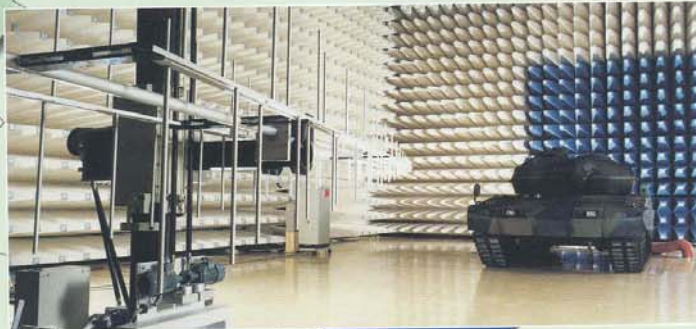
EMC testing of a LEOPARD 2 A6 EX
