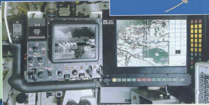
State-of-the-art C 3 I commander's station in the LEOPARD 2
